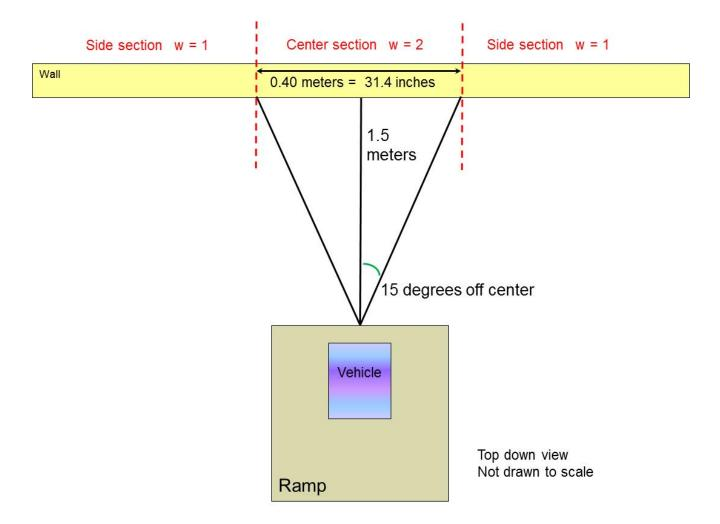
The wall shall be marked with colored tape to indicate the side and center sections. If any part of the vehicle crosses over into the side sections, it will be counted as w=1. The vehicle should not deviate off the center point more than 15 degrees in either direction.
